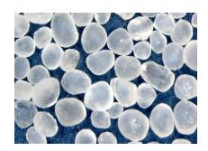
• Meets or exceeds API RP-19C and ISO 13503-2 specifications for particle distribution, roundness and sphericity, turbidity, and solubility
